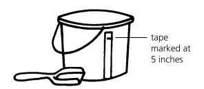
Procedure: On the outside of the bucket, run a strip of masking tape from top to bottom. Set the bucket on the floor and use the marker to mark a point on the tape 5 inches (12.5 cm) up from ground level. Fill the bucket with 5 inches of snow. If possible, scoop freshly fallen snow from an undisturbed spot. Take the bucket inside and let the snow melt. Mark the water level on the tape. Measure from ground level as before to determine the amount of water in 5 inches of snow.
